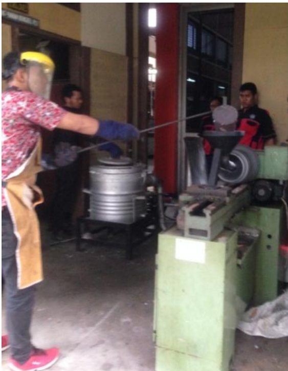
Fig. 5. Centrifugal casting process
